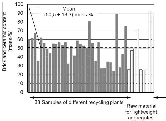
Fig. 3. Brick content of 42 masonry samples taken from processed masonry rubble piles at various stationary recycling plants including the used raw materials (own results).
