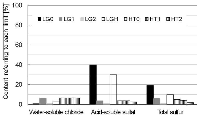
**Fig. 14.** Content of chloride, sulfate and total sulfur of various lightweight aggregates referring to the relevant limits that are set as 100% (LG: lightweight aggregates produced in the laboratory; HT: lightweight aggregates produced by small-scale manufacturing).
