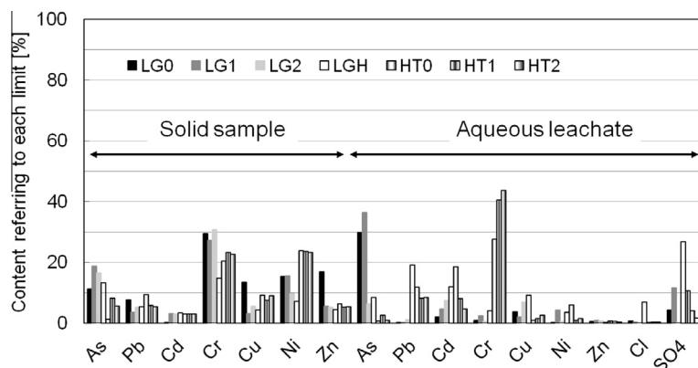
**Fig. 15.** Content of arsenic, heavy metals and salts of the solid sample and the aqueous leachate (batch test with liquid/solid ratio of 10 to 1 kg) of various lightweight aggregates referring to the relevant limits that are set as 100% (LG: lightweight aggregates produced in the laboratory; HT: lightweight aggregates produced by small-scale manufacturing).
