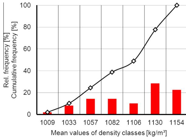
**Fig. 13.** Particle density distribution of the lightweight aggregates from masonry rubble with 48 mass% brick, fired once.
