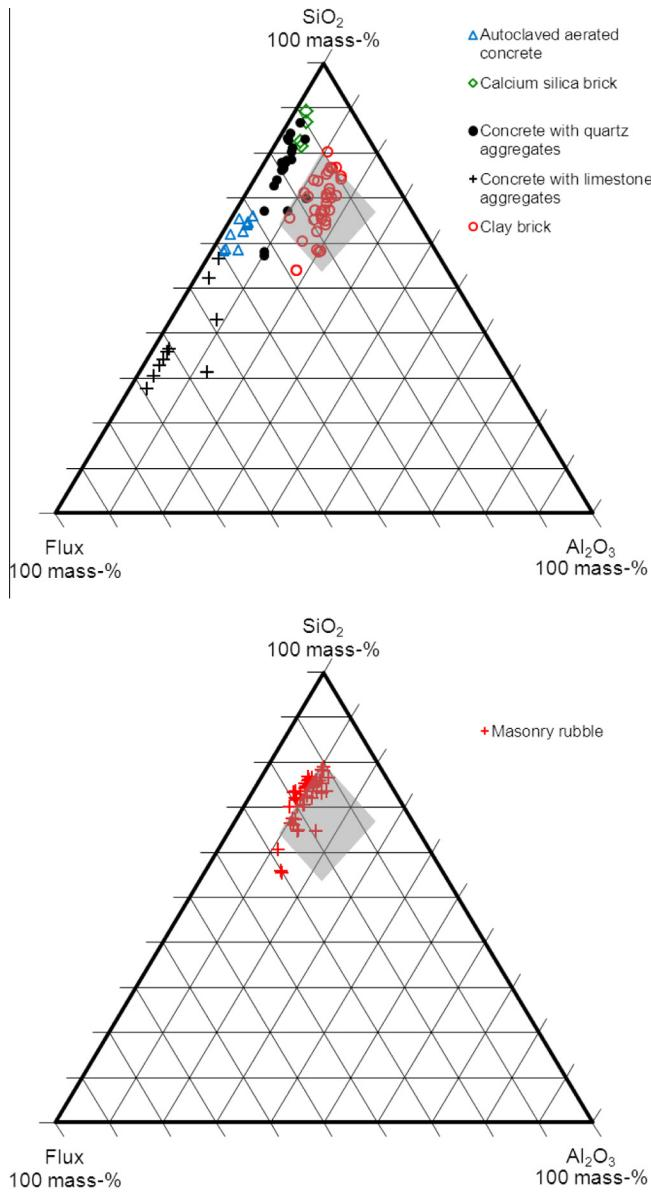
**Fig. 5.** Relative positions of the unmixed main components of masonry rubble and of real masonry rubble in the ternary system  $\text{SiO}_2\text{-Al}_2\text{O}_3\text{-flux}$  ( $\text{CaO} + \text{MgO} + \text{Fe}_{2}\text{O}_3 + \text{Na}_2\text{O} + \text{K}_2\text{O}$ ) Gray area: [22,23]. Data points: own results.
