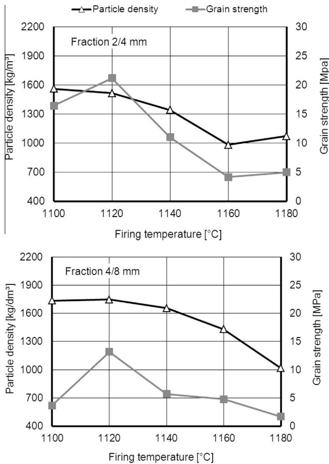
**Fig. 8.** Influence of the firing temperature on the particle density and the grain strength of expanded granules produced from masonry rubble MW 1 with 48 mass% clay brick, dosed with 3 mass% SiC.
