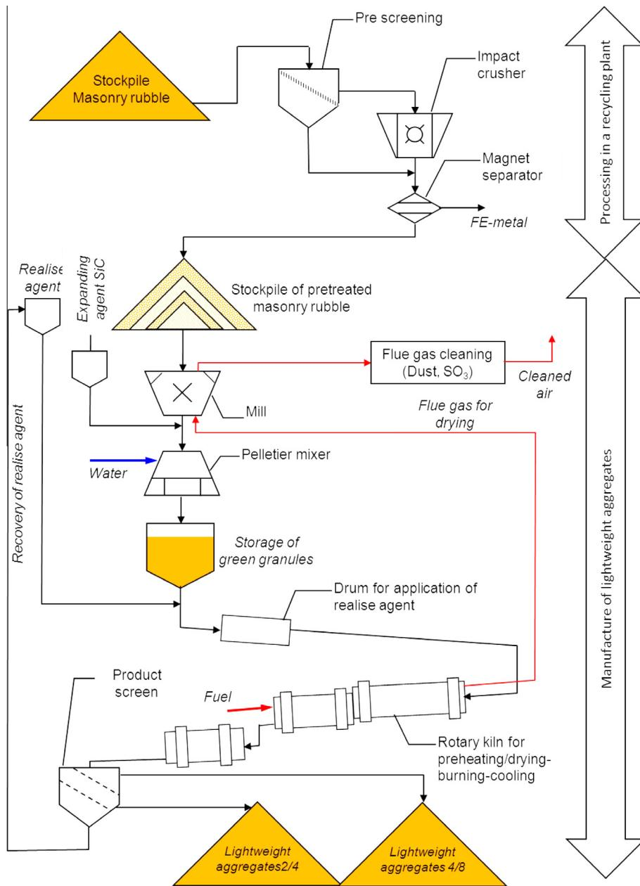
**Fig. 20.** Simplified manufacturing process for lightweight aggregates from masonry rubble.
