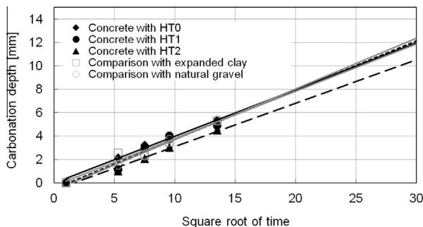
**Fig. 18.** Carbonation of lightweight concretes with different lightweight aggregates from masonry rubble measured at prisms of  $40 \text{ mm} \times 40 \text{ mm} \times 160 \text{ mm}$  stored at  $23^\circ\text{C}$  and 50% relative humidity (HT: lightweight aggregates produced by small-scale manufacturing, comparison concrete with expanded clay and natural gravel).
