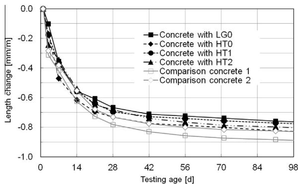
**Fig. 17.** Time dependant shrinkage behavior of different lightweight concretes with lightweight aggregates from masonry rubble measured at prisms of  $40 \text{ mm} \times 40 \text{ mm} \times 160 \text{ mm}$  stored at  $23^\circ\text{C}$  and 50% relative humidity (LG: lightweight aggregates produced in the laboratory; HT: lightweight aggregates produced by small-scale manufacturing, comparison concrete with different expanded clays).
