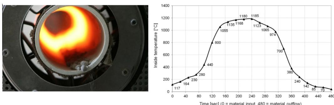
Fig. 7. Kiln outlet and temperature profile in the kiln.
