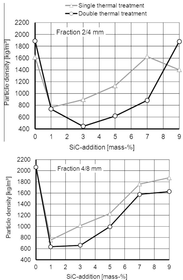
**Fig. 9.** Influence of SiC-dosage on the particle density of expanded granules produced from masonry rubble MW 1 with 48 mass% clay brick, fired at a temperature of 1180 °C.
