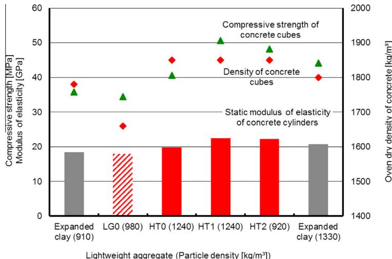
**Fig. 16.** Mechanical properties of laboratory concretes produced using lightweight aggregates from masonry rubble (LG: lightweight aggregates produced in the laboratory; HT: lightweight aggregates produced by small-scale manufacturing).
