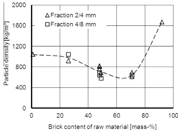
**Fig. 10.** Influence of the brick content of the input material on the particle density of the expanded granules produced from masonry rubble, under the following conditions: SiC-dosage 1 or 3 mass%, firing temperature 1165–1180 °C (values from [25], among others).
