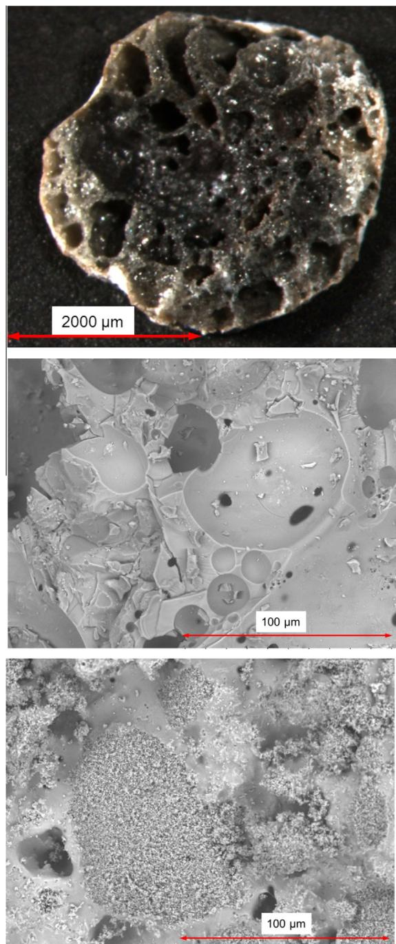
**Fig. 12.** Overview image of the fracture surface of an expanded granule (top) and micrograph of the surface (middle) and the inside (bottom) of the granule. Provided by Alexander Schnell (top), Steffen Liebezeit (middle, bottom).
