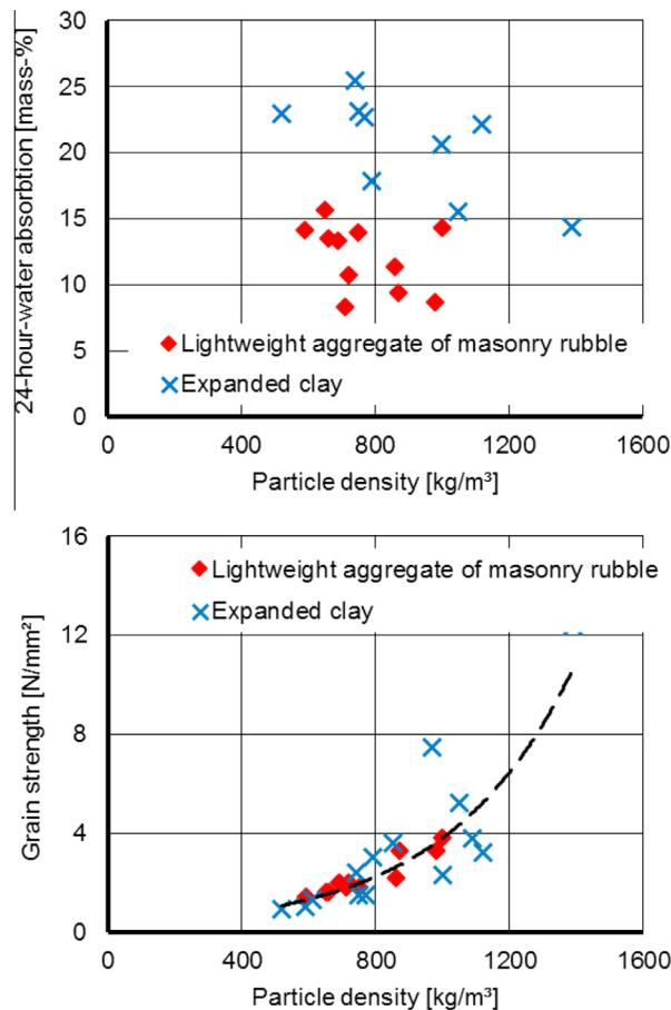
**Fig. 11.** Dependence of water absorption and grain strength on particle density, comparing lightweight aggregates from masonry rubble with expanded clay.
